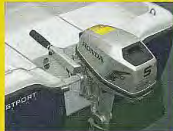
↑ Our test craft was fitted with a tiller-steering Honda BF5p outboard motor.
